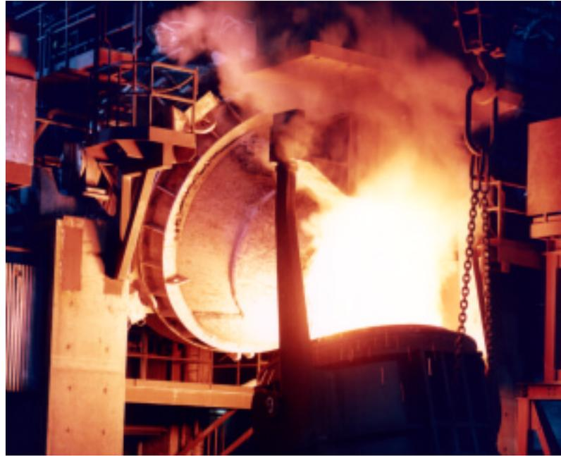
80 Ton AOD pouring heat into crane ladle
