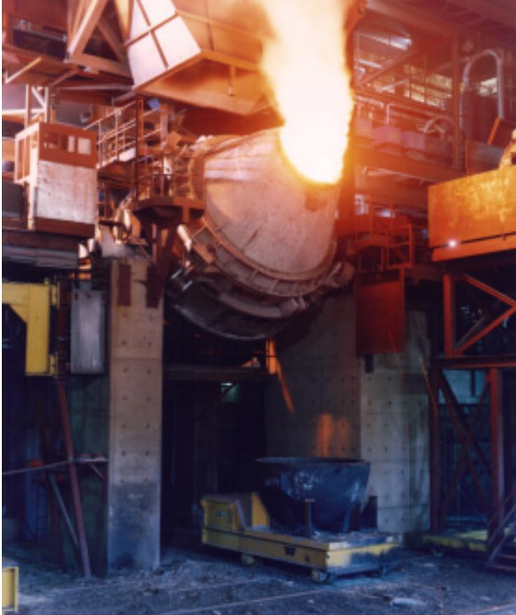
80 Ton AOD preparing to slag off into slag pot transfer car
