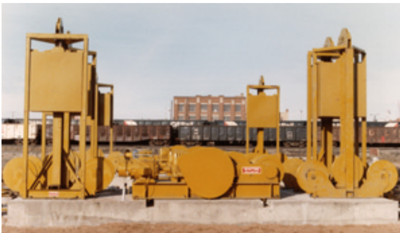
Above and right - Continuous rope pullers, installed with counterweight towers, provide the muscle for Whiting ROBOT Systems.
