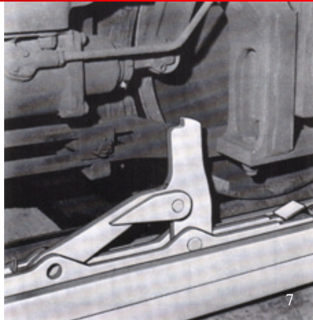
ROBOT arm contacting journal. For use when there are pits, scales, hoppers or other obstructions between rails.
