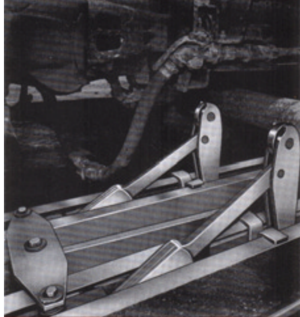
Double arm contacting axle. For draw bar pulls of 35,000 to 70,000 lbs.
