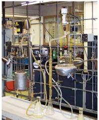
Pilot facilities include a rising film and falling film evaporator, three forced-circulation evaporative crystallizers and two draft tube baffle crystallizers.
