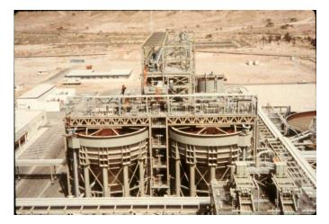
The Draft Tube Baffle (DTB) crystallizer is the most successful of the crystallizers designed to make the large, uniform crystals required for fertilizer and similar applications where superior filtration, centrifugation, washing, drying, and storage characteristics are required. This Swenson design is the result of years of ongoing research and development as well as proven plant operation in many installations.
