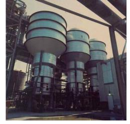
The Falling-Film long-tube vertical evaporator is preferred for heat-sensitive liquors. A film of liquor flows down the inside of a tube and is circulated to maintain the required flow.
