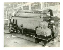
These rotary filters are easy to maintain and keep clean. Because they operate at low speed they have a long service life.
