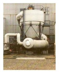
For operation at temperatures below which it is not economically possible to use vacuum equipment, or with solutions with very high boiling point elevations, the Surface-Cooled Crystallizer using a shell and tube exchanger is supplied.
